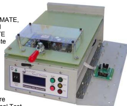
The complete Scorpion test system is highlighted in the block diagram below. The external DMM is controlled by the Pico-MATE and is used to acquire measurements that support both ICT and Functional Test.
